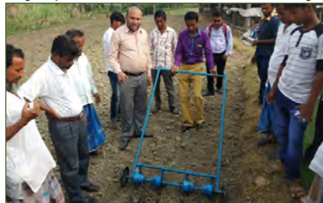
Fig 9.11. Demonstration of CRIJAF Multi-Row Seed Drill under Jute-ICARE programme
