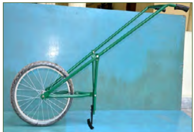
Fig.7.2. CRIJAF Single Wheel Jute Weeder with modified scraper unit
