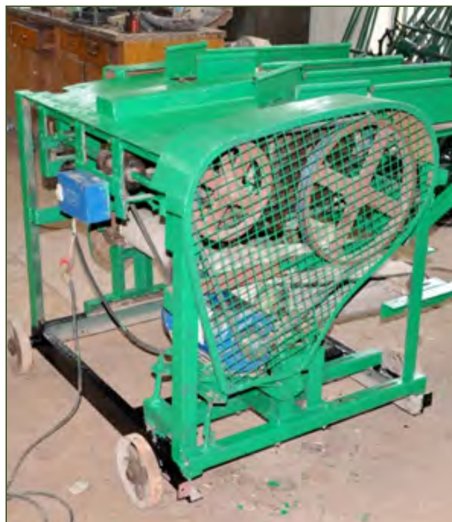
Fig. 7.4. Experimental model of power operated jute ribboner machine
