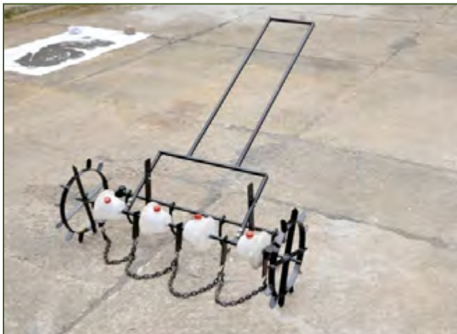
Fig.7.1. Manual operated multi-crop seeder
