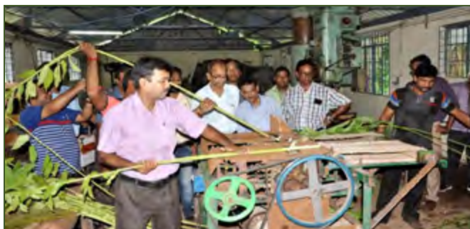
Demonstration of ribbon extraction in workshop
