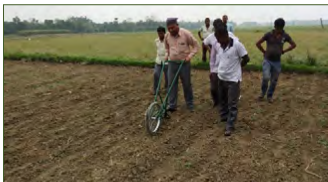
Fig 9.10. Demonstration of CRIJAF Single Wheel Jute Weeder under Jute-ICARE programme
