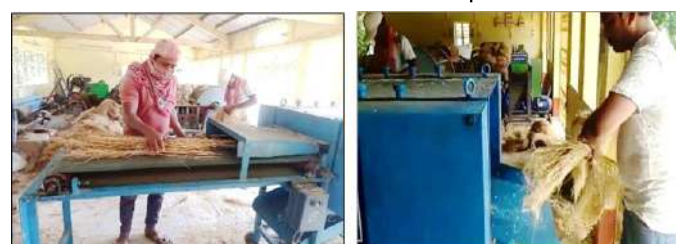
Fig. 15. Extraction of flax fibre using Improved Flax Fibre extractor
