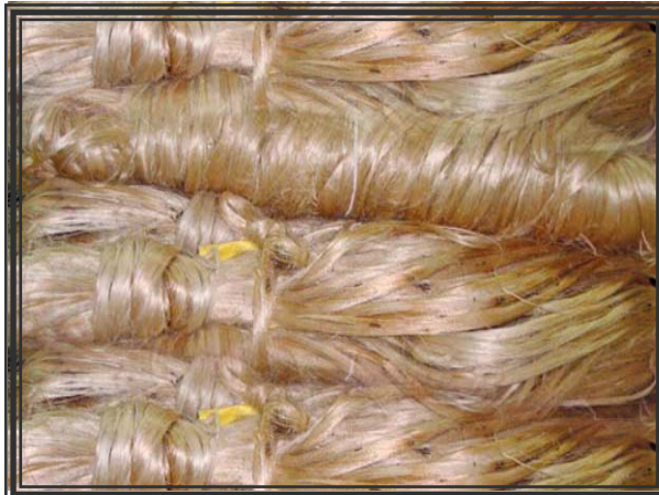
Fig 4. Lustrous fibre obtained through retting of green ribbons using microbial consortium
